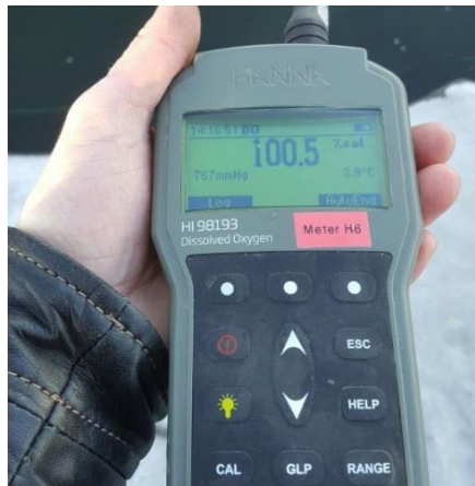
Figure 6-21. Measurement of the dissolved oxygen of the water storage of Proeftuin Zwaagdijk (The Netherlands) where a floating Airlift is installed
