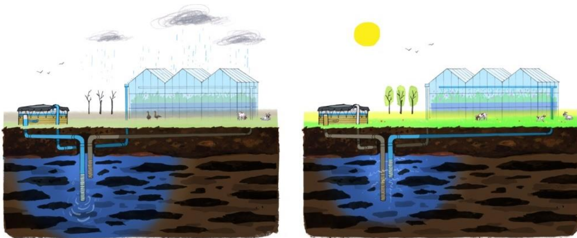
Figure 2-17. Use of aquifer storage and recovery (ASR) in the Dutch greenhouse sector. Rainwater is pre-treated by slow sand filtration and infiltrated in a deep aquifer (sand layer, approximately 10 – 50 m deep)
