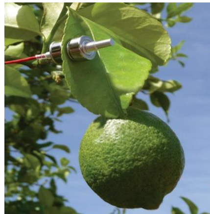
Figure 10-22. Yara water sensor
