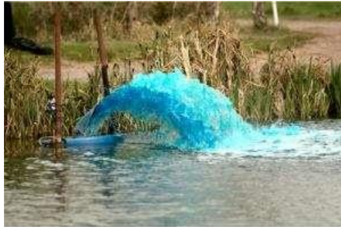
Figure 5-20. Blue dye being dispersed into the water via a pump ( www.dyofix.co.uk )
