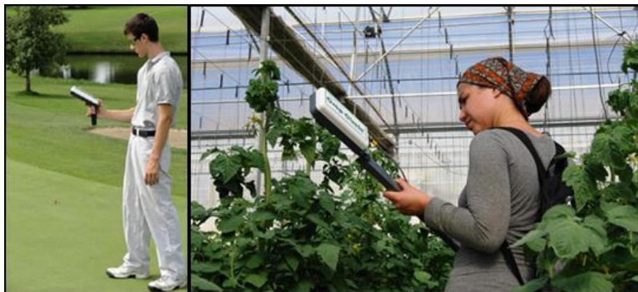
Figure 11-29. Measurements with reflectance sensors
