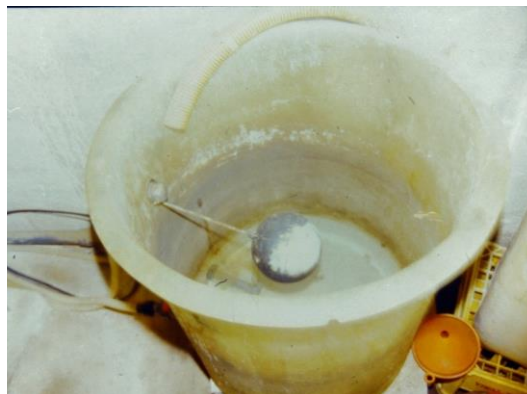
Figure 8-3. Picture of open fertilisation tank connected to the pump aspiration (Source: Juan Carreño Sánchez)
