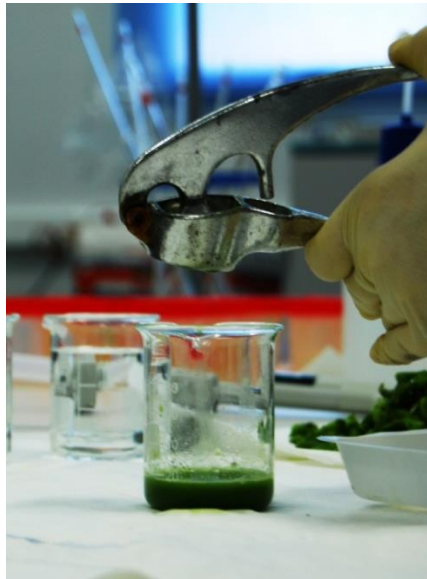
Figure 11-23. Squeezing sap from cut petioles using garlic press
