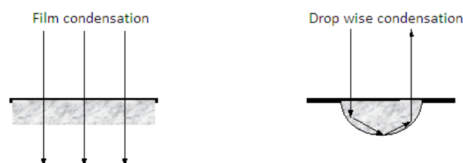
Figure 2-37. Effect of condensation on light transmission
