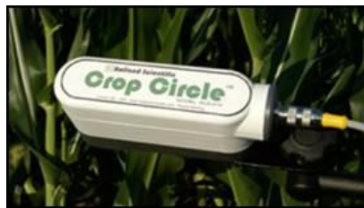
Figure 11-26. A crop circle reflectance sensor
